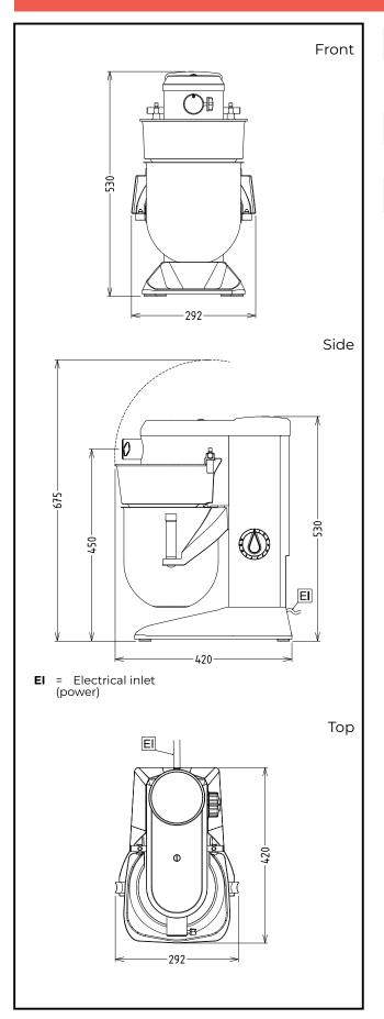
Electric Supply voltage: 200-240 V/1N ph/50/60 Hz Electrical power, max: 0.6 kW **Total Watts:** 0.6 kW Capacity: Performance (up to): 2.5 kg/Cycle Capacity: 8 litres Key Information: External dimensions, Width: 292 mm External dimensions, 416 mm Depth: External dimensions, Height: 527 mm **Shipping weight:** ISO 9001; ISO 14001 kg Net weight (kg): **Cold water paste:** 2.5 kg with Spiral hook
